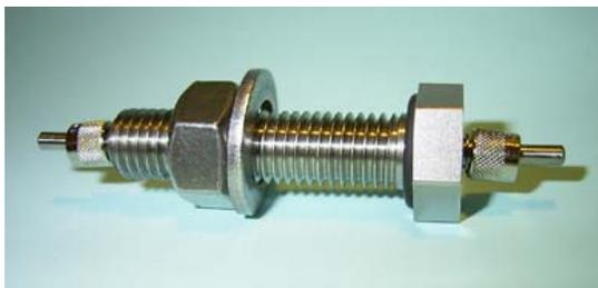
The FC-VFT vacuum feedthroughs are designed for use of fiber optics in vacuum chambers, such as for plasma monitoring. The vacuum feedthrough consists of an M12 housing with Viton® O-ring and 2 SMA fiber optic interconnects to allow easily coupling to fiber optic cables and probes. The vacuum feedthrough can be delivered for all fiber diameters, such as 50  $\mu\text{m}$  up to 1000  $\mu\text{m}$  for UV/VIS as well as for VIS/NIR. (This is a product of Avantes, Inc., Boulder, Colorado.)
